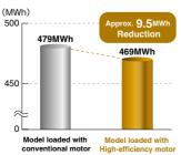
Calculation Condition: 415V/50Hz, Air Compressor Load Ratio at 90%, 6.000h/vear Operation Time. Except auxiliary equipment
